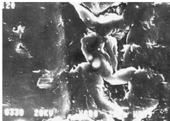
Figure 2 SEM photograph of the abraded surface of UHMWPE against quartz sand of size 0.420–0.840 mm at the sliding velocity of 2.35 m/s.
